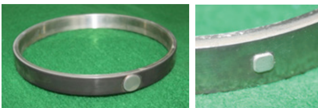
图4 旋印电解加工工艺加工出的典型凸台 Fig.4 Typical boss manufactured by rotary printing ECM
